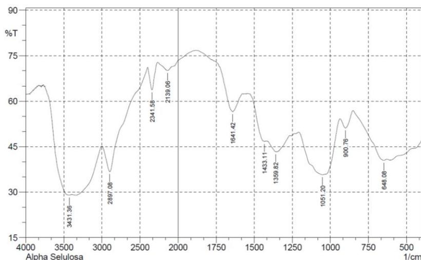
Fig 1. FT-IR Spectrum – Cellulose from Oil Palm Empty Fruit Bunches
