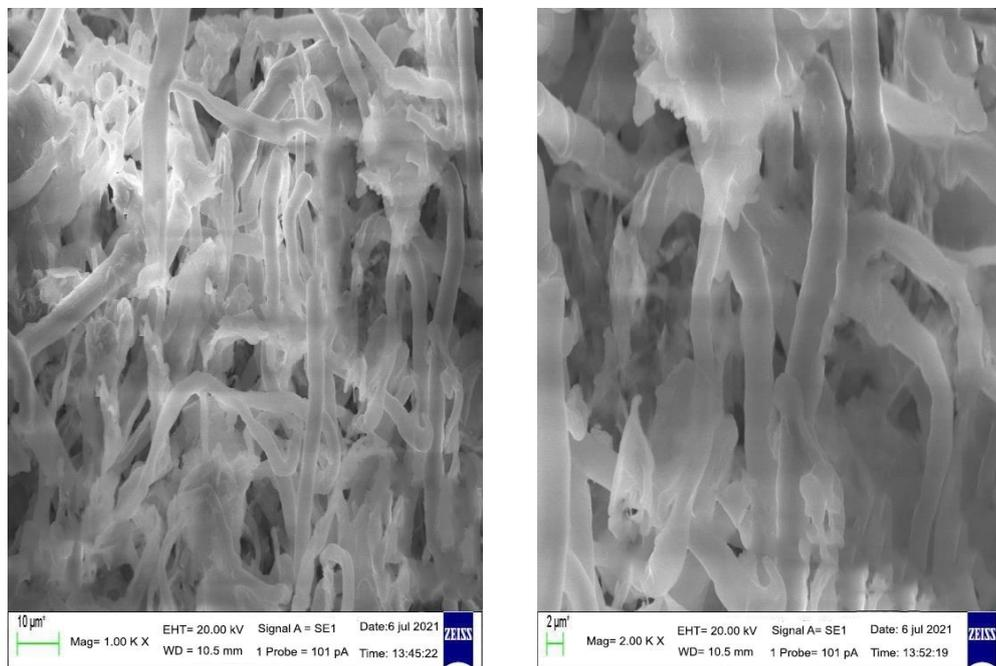
Fig 5. SEM results of cellulose stearate ester (a) 1000x magnification (b) 2000x magnification
