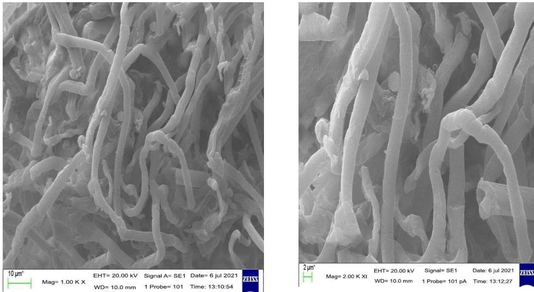
**Fig 2.** SEM results of -cellulose EFB (a) 1000x magnification (b) 2000x magnification
