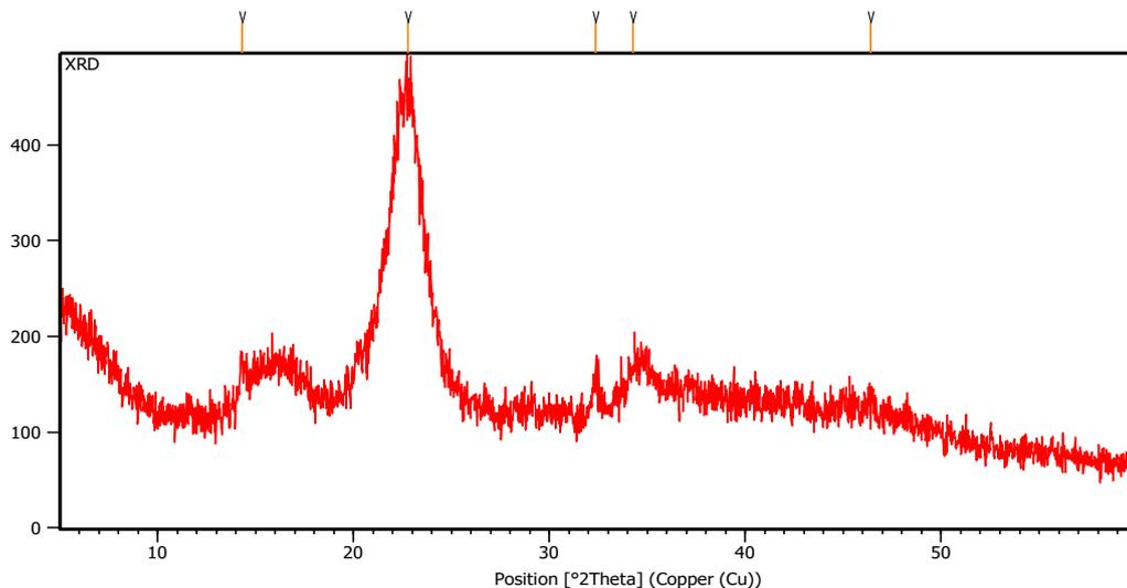
**Fig 6.** Cellulose Stearate XRD test results
