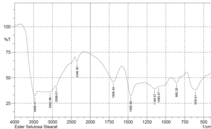
**Fig 3.** Cellulose Stearate Esters FTIR Spectrum
