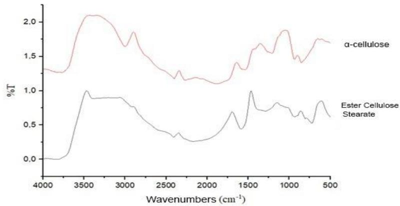
Fig 4. Comparison of FTIR Spectrum of Cellulose and Cellulose Stearate
